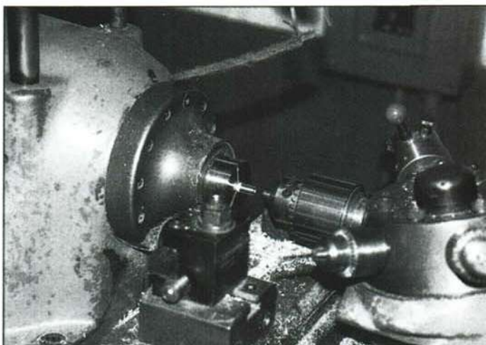
Drumstick cores are threaded by means of a precision tip-machining operation.
